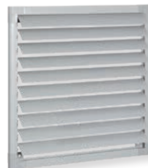
The PVC shutters adjust automatically and close when the fan stops.
