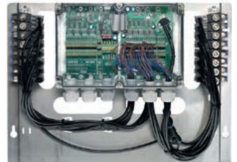
Valve cluster for pneumatically actuated feed valves
