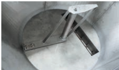
Hopper bottom with Z-shaped blade and discharging auger
