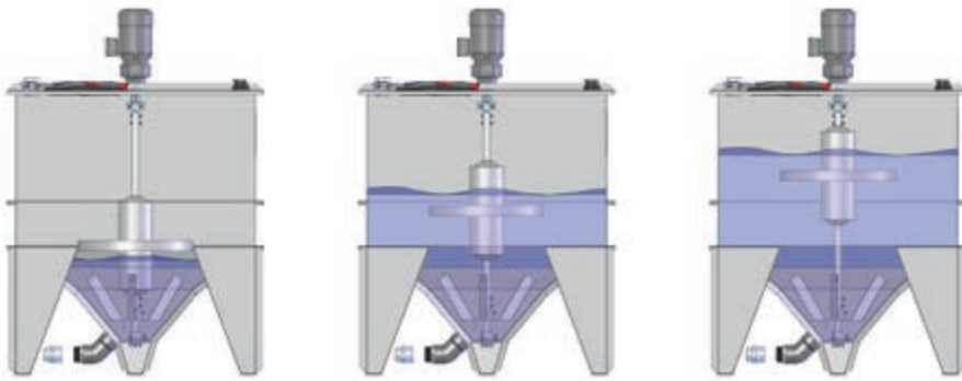
How the level-controlled agitator works (schematic view)
