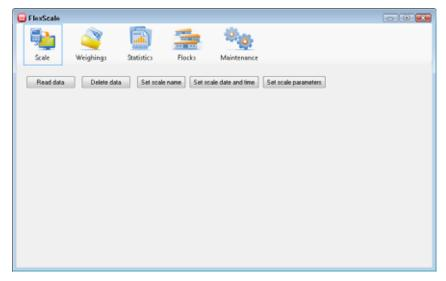
Click the *Read data* button. A dialog will display notifying you to wait and all data will be downloaded from the scale. The communication with the scale may last several minutes depending on the amount of data. When completed, a table with all weight data will be displayed.
