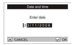
Enter the correct date using keys  $\bigcirc$ ,  $\bigcirc$ ,  $\bigcirc$  and  $\bigcirc$ . After pressing  $\bigcirc$  the time setting dialog box displays. Enter the correct time using keys  $\bigcirc$ ,  $\bigcirc$ ,  $\bigcirc$  and  $\bigcirc$ .
