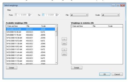
The left list includes all available weighings sorted by date. The right list includes weighings selected in the statistics. Select a row in the *Available weighings* table and click the > button. You can repeat the procedure several times. Close the dialog by clicking *OK*. Selected weighings will be displayed in the table, where you can see and compare their statistics, histogram, and individual weights.
