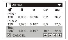
If the mode of weighing with the sex selection is activated, use keys  $\bigcirc$  and  $\bigcirc$  to display the statistics for cocks and hens.
