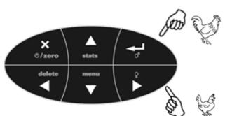
The weight displayed at the time of pressing the key is saved into the file, including the selected sex. Now remove the bird from the hook and continue with next bird.
