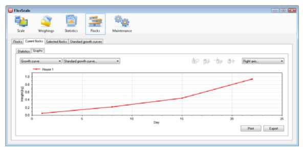
The horizontal axis specifies the flock age and the vertical axis specifies the average weight of the flock.
