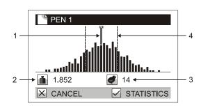
Press or to move the cursor to any weight column; the weight and the number of birds represented in this column will be displayed below the graph. Press the key to continue weighing.
