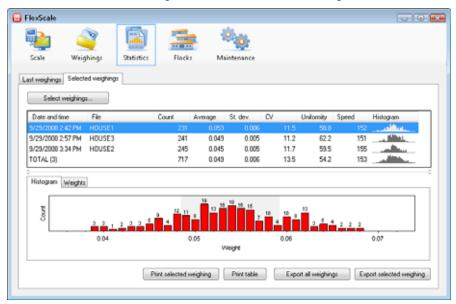
You can print the selected row of the statistics including the histogram by clicking the *Print selected weighing* button. You can print the statistics table as it is displayed on the screen using the *Print table* button.
