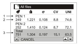
Use the \(\overline{\text{\text{\text{e}}}}\) key to display the next page. Use the \(\overline{\text{\text{\text{c}}}}\) key to display the previous page. If the mode of weighing with sorting is activated, use keys \(\overline{\text{\text{c}}}\) and \(\overline{\text{\text{c}}}\) to display statistics for light, acceptable and heavy birds.
