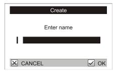
Using keys  $\bigcirc$ ,  $\bigcirc$ , and  $\bigcirc$  enter the name of the group and press  $\bigcirc$ . A list of files is displayed; use the  $\bigcirc$  key to select files that belong to the group.
