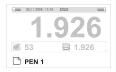
Now you can weigh individual birds from Pen 1, as described in Chapter 3. An incorrect weight can be deleted by pressing the  $\bigcirc$  (DELETE) key. A confirmation will be displayed.
