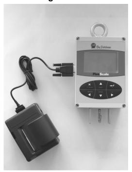
Connect the printer cable into the DB9 serial port on the scale and switch the printer on.
