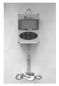
Suspend the scale using a chain on a firm, non-spring biased structure. Place a hook on the scale and switch the scale on by pressing the  $\boxtimes$  key.
