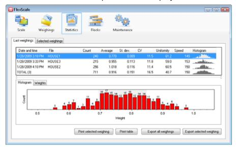
Files that have just been downloaded from the scale will be displayed in the table. The histogram will be displayed in the lower half of the panel for the highlighted file. Individual weights in this file will be displayed after clicking the *Weights* tab.
