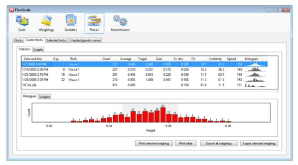
The rows in the table show individual days when the flock was weighed. The histogram for the selected day is displayed in the lower half of the panel for the highlighted row. Individual weights weighed for this day will be displayed after clicking the *Weights* tab. Select the *Graphs* tab to monitor the flock progress in a graphic form.
