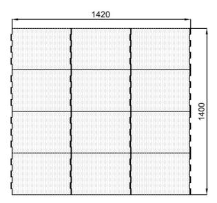
Figure 6-9: StuffNix V15 short version: 4 x 3 basic elements = 1 filter element
