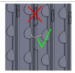
Figure 6-26: Mounting clamps on basic elements
