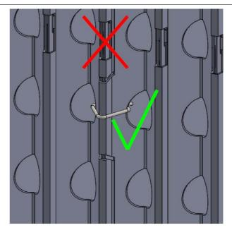
Figure 6-17: Clamp mounted on basic elements
