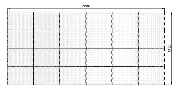
Figure 6-8: StuffNix V15: 4 x 6 basic elements = 1 filter element
