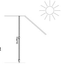
Figure 3-8: Protecting StuffNix V15 from direct sunlight
