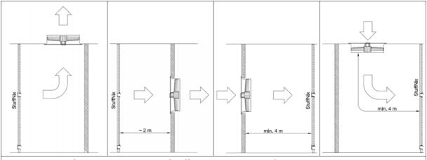
Figure 3-7: Options to arrange StuffNix V15 and the fan
