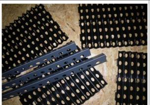
Figure 6-10: Individual filter parts
