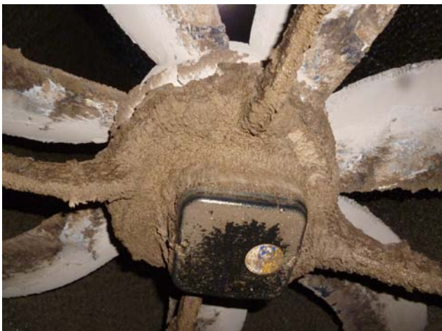
Fig. 1 & 2: Exhaust air fans of a MagixX-L after longer operation
