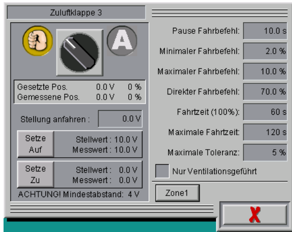
Figure 7-7: Analogue intake air flap with feedback
