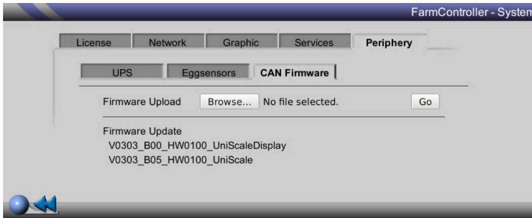
Figure 4-29: CAN modules: uploading new firmware
