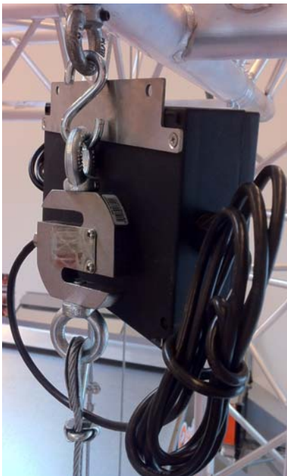
Fig. 2: Swing weigher with converter at the ceiling hook
