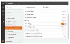
Preheating ensures that the inside temperature does not fall below the set temperature when batch status is empty house for a longer period of time.
