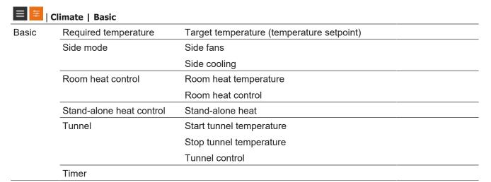
The **Basic** menu gives you access to setting of each side and tunnel fan and each house and stand-alone heater by means of matrix menus.
