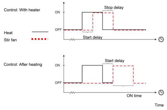
Figure 6: Control with heater
