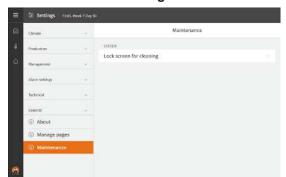
When the controller is to be cleaned, it is possible to lock the screen to avoid inadvertent operation during cleaning. Lock the screen in the menu [Secretary | General | Maintenance | Lock screen for cleaning.]
