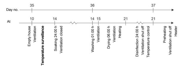
Figure 9: Sequence of in-between functions
