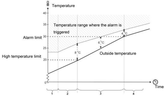
Figure 11: Summer temperature at 20° C and 30° C outside
