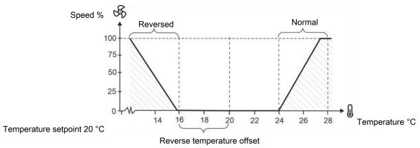
Figure 5: 0-10 V-controlled stir fan with reverse relay
