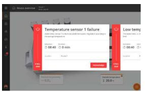
When an alarm occurs, the house controller will register the alarm type and the time it occurred.
