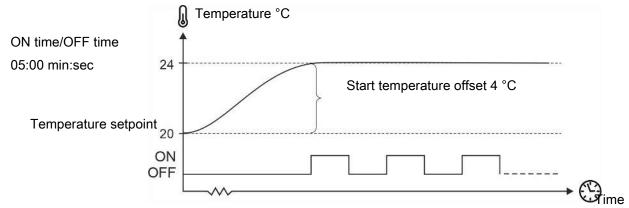
Figure 3: Relay-controlled stir fan (ON/OFF) controlled by temperature
