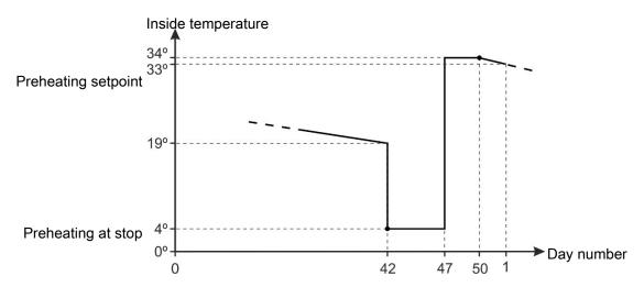
Figure 10: Example of setting of preheating.
