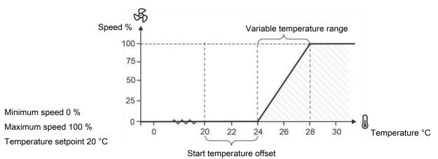
Figure 4: 0-10 V controlled stir fan with a positive Start temperature offset.
