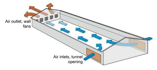
Figure 1: Tunnel ventilation principle
