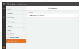
When the controller is to be cleaned, it is possible to lock the screen to avoid inadvertent operation during cleaning. Lock the screen in the menu [ General | Maintenance | Lock screen for cleaning.
