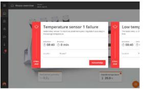
When an alarm occurs, the house controller will register the alarm type and the time it occurred.
