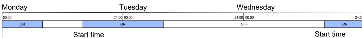
Figure 12: If an ON-time runs past midnight on a day when the 24-hour clock is not active, the function will remain ON until the time has elapsed.
