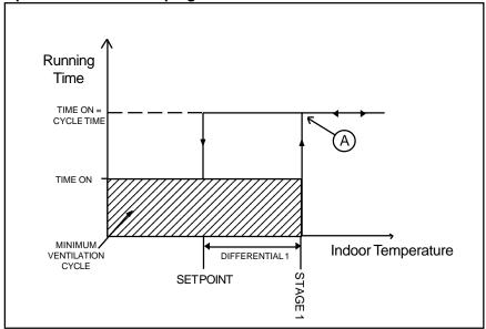
This option is activated when ramping is turned off. When the temperature is less than the set point + differential 1, Stage 1 fans run according to the minimum cycle (see above). When the room temperature reaches point A, stage 1 fans run continuously with no transition.
