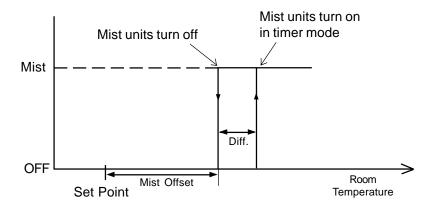
The mist units operate according to a timer cycle. Time on is the running time of the mist units and time off is the off time of the mist units.
