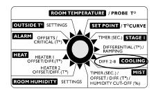
Press the push-button. The current differential for Stage 3 flashes on the display, alternating with the letters "St 3".
