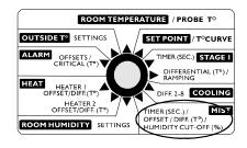
Press the push-button three times. The mist differential is displayed, alternating with the letters "**dIF**",
