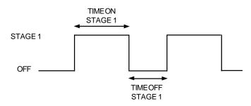
During time on, the Stage 1 fans run. The Stages 1-2 Pilot Light flashes. During time off, the Stage 1 fans do not run. The Stages 1-2 Pilot Light turns off.
