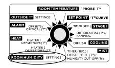
Turn the adjustment knob clockwise one notch further. The maximum humidity flashes on the display, alternating with the letters "**Hi**".
