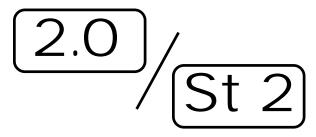
(ii) If, after about 6 seconds, no action is taken by the user, the absolute temperature value is displayed, alternating with "St 2" and "Str". In this case, the absolute value is: Set Point + Stage 1 Differential + Stage 2 Differential.
