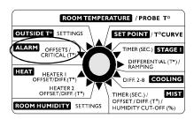
Use the adjustment knob to set the low alarm offset to the desired value.
