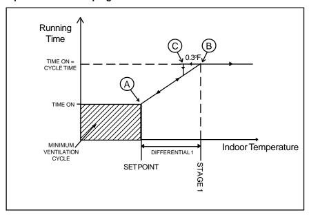
This option is activated from the front panel. At room temperatures at or below the set point, the controller operates the Stage 1 fans according to the minimum ventilation cycle.
