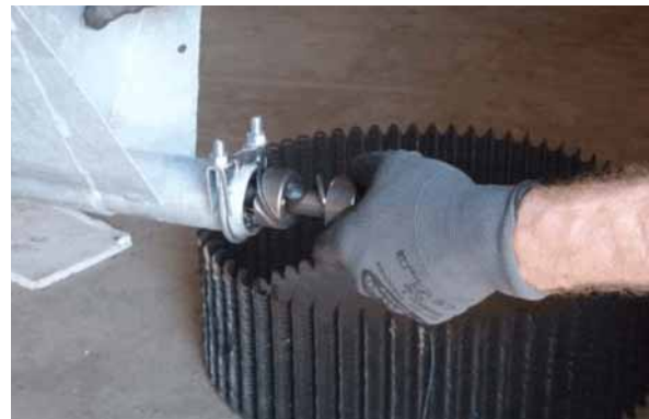
Figure 6-3: Pull out tension shaft
