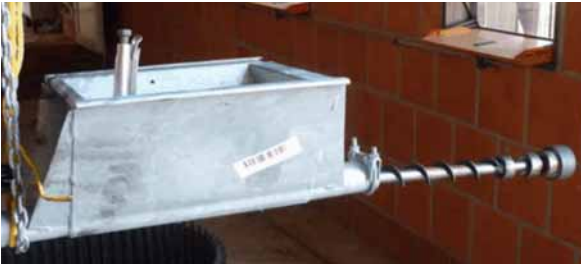
Figure 6-4: Fix the auger by means of a vis-grip wrench
