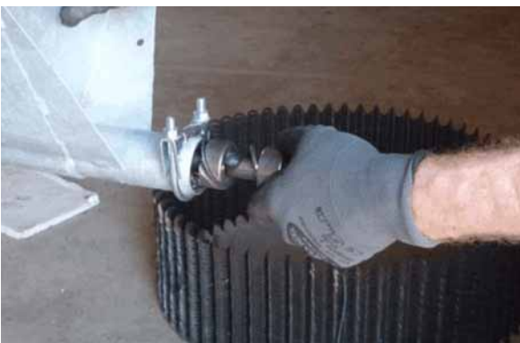
Figure 6-8: Hold the tension shaft
