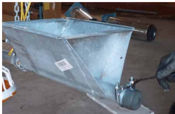
Figure 6-9: Fasten the tension shaft
