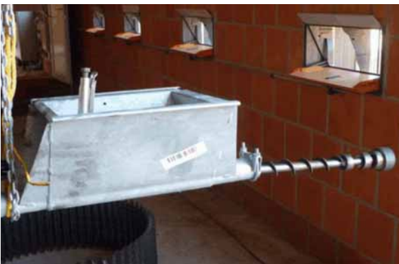
Figure 6-6: Auger to tension shaft
