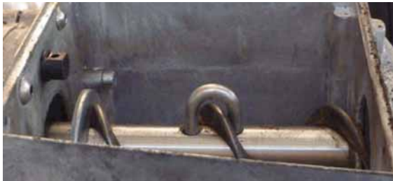
Figure 6-1: Mount the auger on the drive
