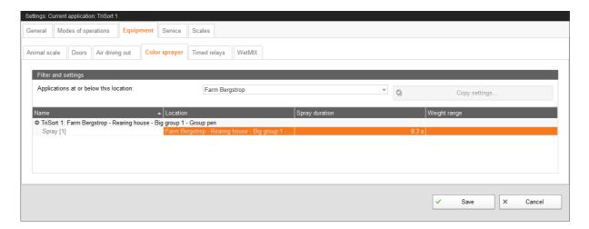
You can control the amount of color used by means of the **spray duration**.
