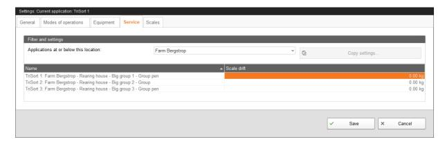
The **Service** function controls the scale. The scale is tared after each weighing and the zero value is reset. If there is a drift, this is registered. The **scale drift** indicates the difference between the zero value during calibration and the current zero value. If the difference exceeds 3 kg, check whether anything affects the weighing process, e.g. dirt. Clean the scale and re-calibrate.
