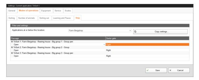
Define whether the entrance and exit door (**Passage**) should remain open or closed if the system has been stopped, and define the position of the sorter gate.
