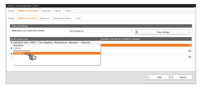
Define under **Modes of operation > Number of animals** whether TriSort is operated with the Pig Manager (Finishing Manager) or not; or whether an external management system is available. The number of animals can be entered manually only in case of operation without Pig Manager.
