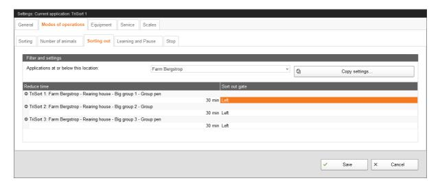
For sorting out, define with the **reduce time** after how much time the start weight is reduced by 1 kg. Also define the position of the **sort-out gate**.
