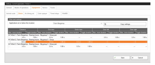
After activation of a door, the door's final position (completely open / closed) must be reached within the **maximum move duration**. Sensors check each door's final position. If the door does not reach its final position within the maximum move duration, it returns to its original position for the time set under **Toggle duration**.
