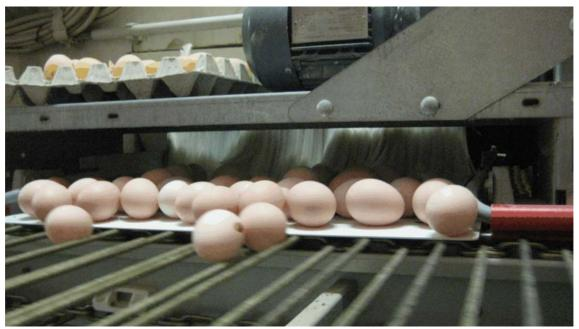
Figure 4-3: Transfer from nest to cross conveyor
