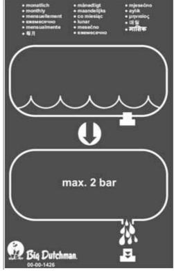
• Check whether the plug for the condensation drain has been inserted.
