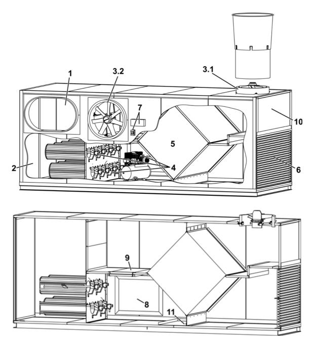
Figure 3-1: Components of the heat exchanger
