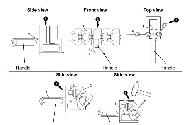
5. Change the length of the chain by removing or adding chain links until it has the correct length.
