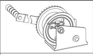
Figure 9-1: Cable fixing for one cable
