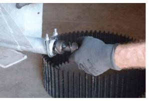
Figure 6-22: Loosen U-bolt
