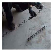
After the inspection for damages, the ends of the auger have to be smoothed off. This is done to make it easier to push the auger into the Augermatic tube.
