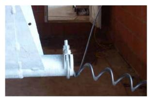
As soon as the auger has its natural tension, it is marked at the outlet of the *lower part for feed hopper* (for example by means of a cable strap Figure figure 6-11).
