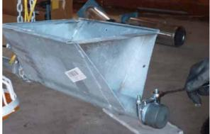
Figure 6-20: Fasten the tension shaft
