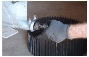
Figure 6-28: Hold the tension shaft
