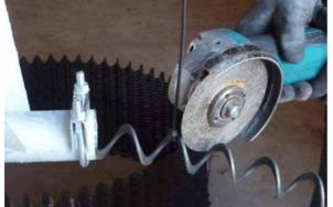
Figure 6-15: Cut off auger
