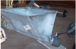
Figure 6-29: Fasten the tension shaft
