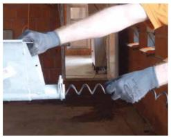
Now the auger has to be pulled out of the *lower* part for feed hopper several times and be released so that it achieves its natural tension and position over the entire length.
