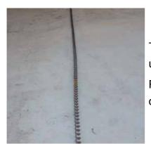
The auger should be checked once again after the uncoiling concerning possible bends and damages. Remove damaged auger pieces and weld the auger once again at this spot (6.2.5 "Weld the auger HD AM").
