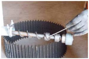
Figure 6-27: Fix auger
