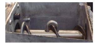
Figure 6-9: Fix the auger to the drive
