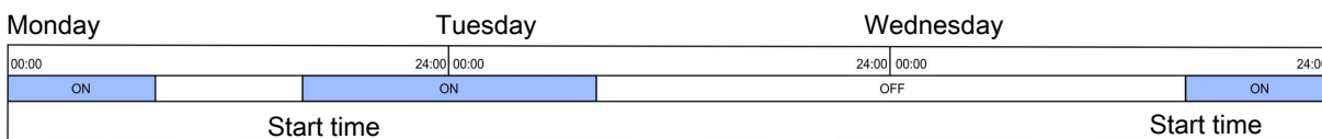
Figure 45: If an ON-time runs past midnight on a day when the 24-hour clock is not active, the function will remain ON until the time has elapsed.
