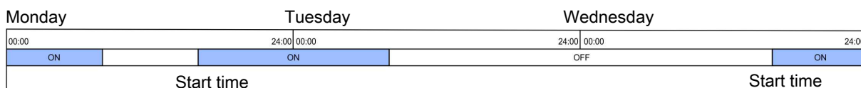
Figure 13: If an ON-time runs past midnight on a day when the 24-hour clock is not active, the function will remain ON until the time has elapsed.
