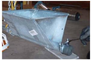
Figure 5-9: Fasten the tension shaft
