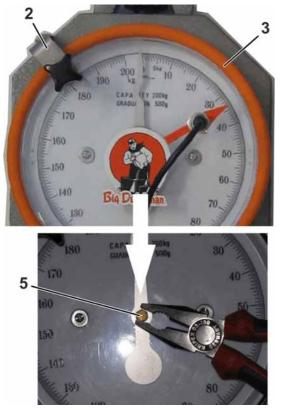
2. Adjusting the desired feed quantity
