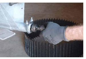
Figure 5-3: Pull out tension shaft
