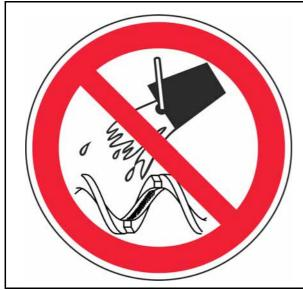
Let the auger **slowly cool down at the air**. A cooling with any liquids makes the material of the auger brittle and thus increases the risk of fracture!
