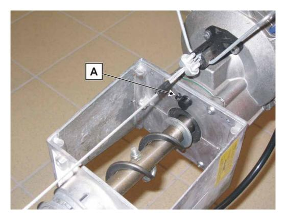
A= Plug for gear aeration is open
