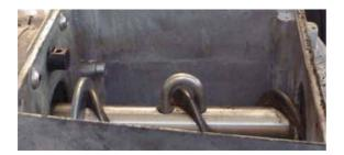
Figure 5-1: Mount the auger on the drive
